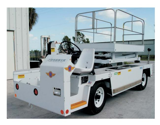
The CMHLM15 is an aerial platform and airport mobile maintenance platform. It is an economic self contained hydraulic platform that is mounted on a manufactured chassis. It has a 15' vertical height and a 20' working height.
