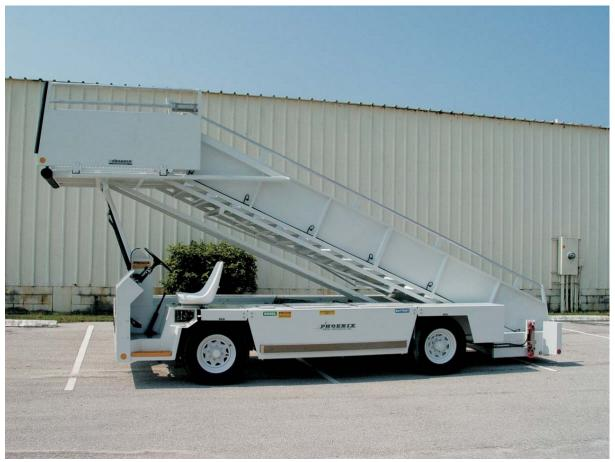
The Phoenix CMPPS96/150 is a chassis mounted, passenger, parallelogram stair. It is designed for the rugged nature of airport ramp operation. The chassis is a heavy duty formed chassis. The stair is a parallelogram design and is made of structural aluminum..
