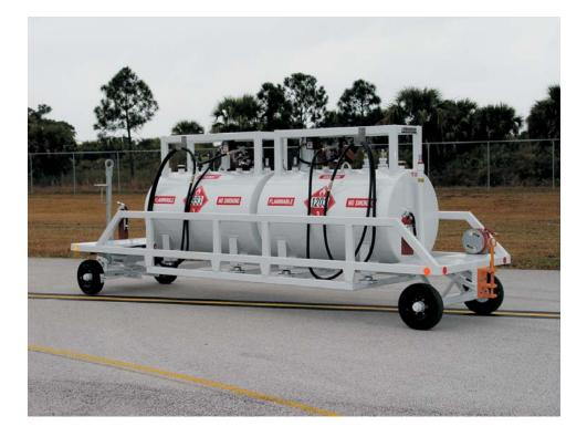
The Phoenix Metal Products, Inc FSC300-2 is a fuel servicing cart for Diesel and Jet A fuels, with (2) 300 gallon-double wall construction tanks. Both tanks have separate pumps, meters, filters and emergency
