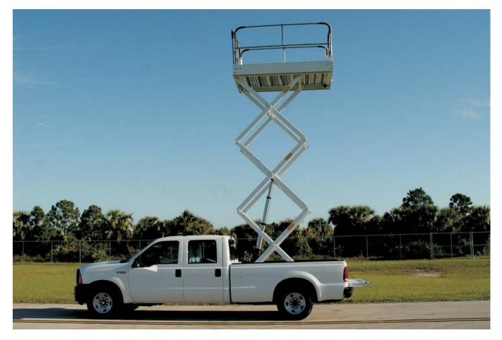
The Hylifter HLM-19 aerial platform and airport mobile maintenance platform is an economic self contained hydraulic platform that fits in a one ton pickup bed and provides 19' vertical height and 25' of working height. The HLM-19 can be supplied as a kit for installation and is as easy as drilling (4) holes and hooking up the furnished recharge isolator.
